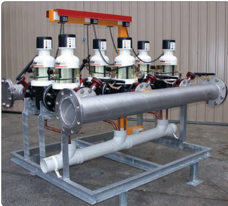
Skid mounted system with six DN100 units
